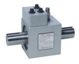
MCRT® 48200V Compact Digital Torque Transducers have high accuracy, low noise, high overload capacity, high overrange, inherent noise tolerance and a wide temperature range. Strain gage sensing and non-contact signal transfer make them well suited for control, laboratory and production use. click for specifications
